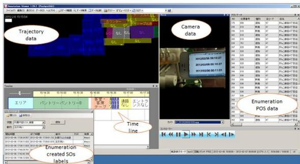
Figure 3 : The service-process analysis support system's main screen
