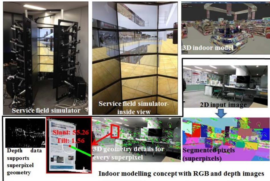
**Fig. 1.** Outlook of the service field simulator with 40 LCD displays, featuring the 3D indoor model. The 3D geometry detected for every superpixel is shown with red dot and green line.
