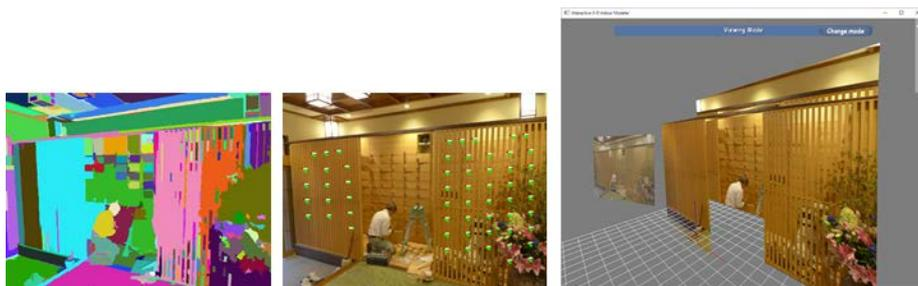
**Fig.5.** Algorithm integration in the 3D modeling. Figure shows the superpixel, the surface normal detected by the algorithm and the orientation guidance for the 3D modeling process.
