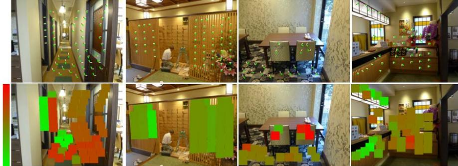
**Fig.4.** Top row: Needle diagram shows the estimated normal (green lines) and the ground truth normal (white lines). Bottom row: Corresponding heatmap; Green zone represents less difference between the normals; More red more deviation from the ground truth.
