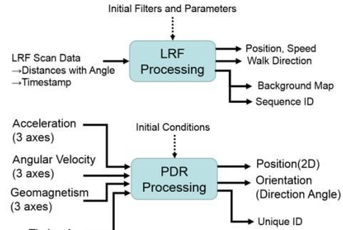
Figure 5: Characteristics of LRFs and PDR
