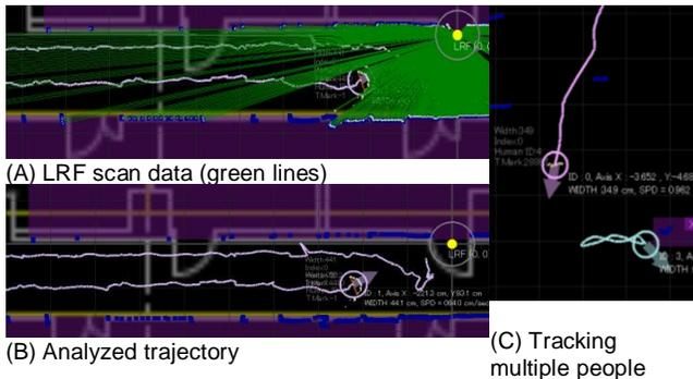
Figure 4: LRF scan data and analyzed trajectories
