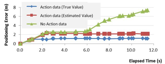
Figure 2: Examples of transition in positioning data error
