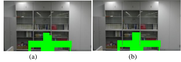
Fig. 11 Comparison between the normal Exemplar-based inpainting and the proposed superpixel based structure propagation (a) Inpainted region for the first iteration in Exemplar-based method (b) Inpainted region for the first iteration in superpixel based structure propagation
