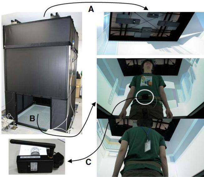
Figure 1. Schematic diagram of WTS: (A) multi-projector, (B) virtual scene displayed around viewer in WTS, and (C) sensor module.
