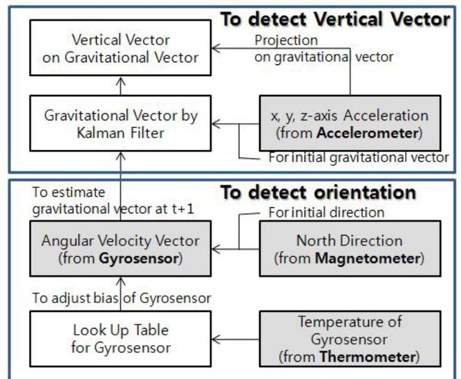
Figure 3. Flowchart to detect WIP and orientation using sensor module.
