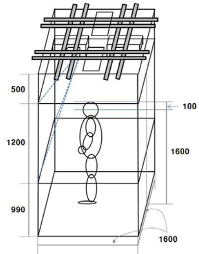
Figure 2. Design drawing of configuration of the proposed WTS.
