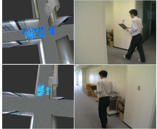
Figure 5. Map matching using a map converted from a 3D environment model (Left-column presents probability distributions of locations of the user shown in right-column. Bottom-row presents the state 1 second before top-row).
