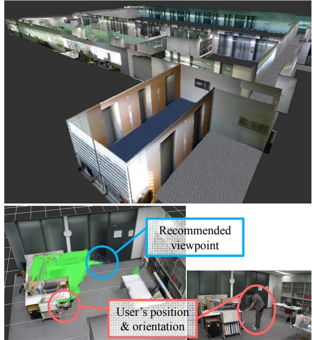
Figure 4. Example of 3D environment model (top) and location-based 3D modeling (bottom). A user can understand shooting position to capture untextured regions by visualization of the recommended viewpoint and own position and orientation. .
