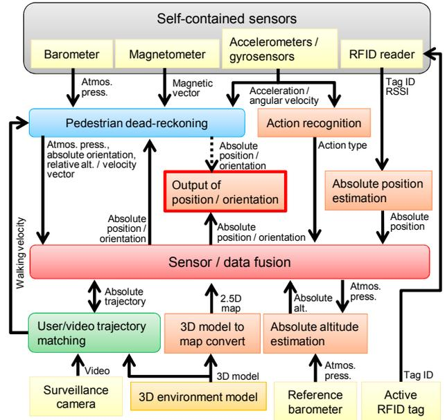
Figure 3. Overview of sensor/data fusion using existing infrastructure and 3D environment model for indoor pedestrian tracking.
