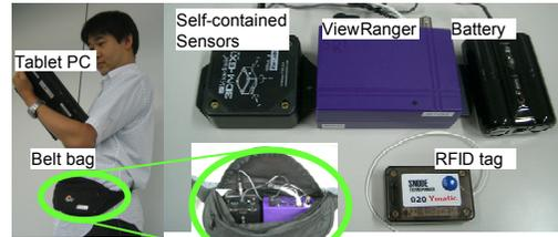
Figure 1. Mobile MR System Hardware Configuration
