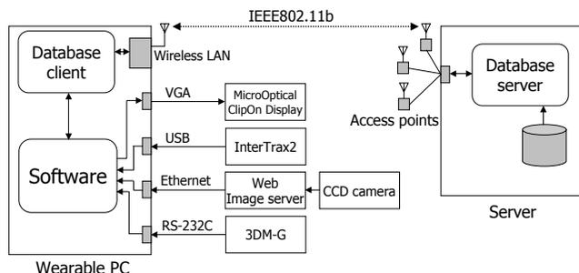
Figure 2: Diagram of personal positioning system.
