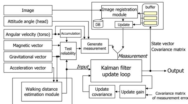
Figure 1: System diagram of the Kalman filter.
