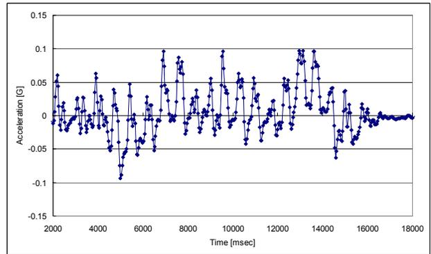
Figure 16: Unfiltered vertical acceleration while in descending elevator in Figure 15.
