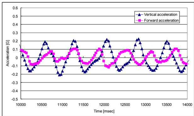
Figure 14: Typical pattern of vertical and forward acceleration while going up stairs.
