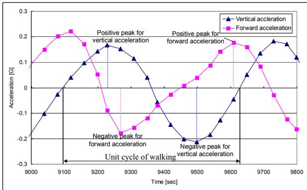
Figure 4: Analysis of unit cycle of acceleration.
