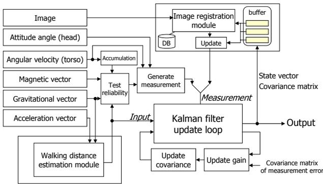
Figure 18: System diagram of the Kalman filter.
