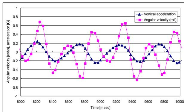
Figure 11: Typical pattern of vertical acceleration and angular velocity (roll-axis) while walking on flat floor.
