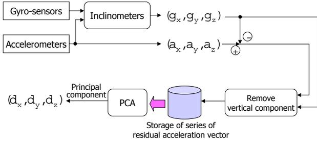
Figure 6: Diagram to estimate forward-and-backward direction.
