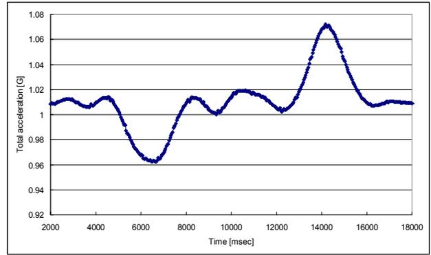
Figure 15: Example of vector length of aggressively low-pass filtered vertical acceleration vector while in descending elevator.
