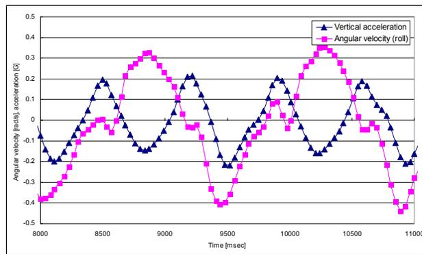
Figure 10: Typical pattern of vertical acceleration and angular velocity (roll-axis) while going up stairs.
