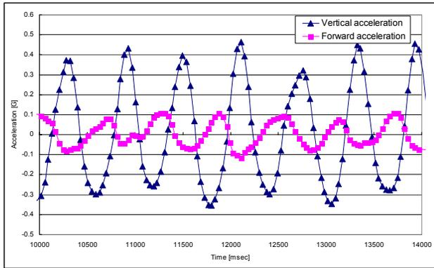
Figure 13: Typical pattern of vertical and forward acceleration while going down stairs.
