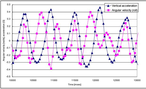
Figure 12: Typical pattern of vertical acceleration and angular velocity (roll-axis) while going down stairs.
