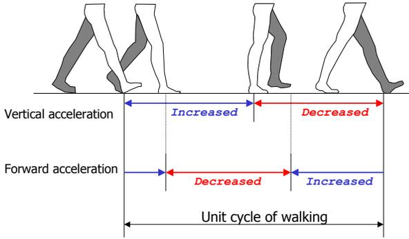
Figure 3: Walking stage and acceleration pattern.
