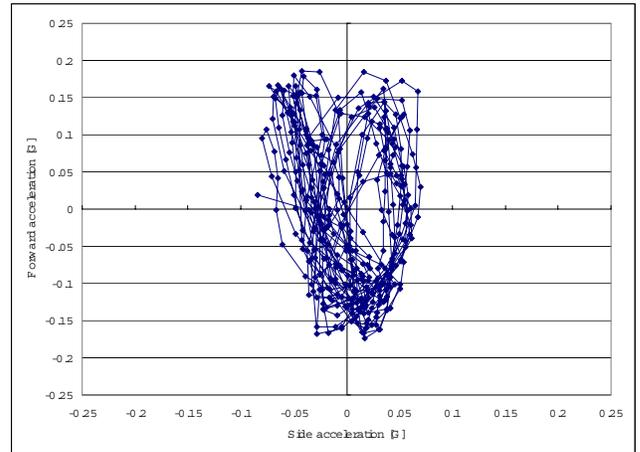
Figure 5: Typical distribution pattern for side and forward acceleration.
