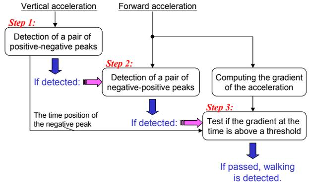
Figure 7: Diagram of detecting unit cycle of walking.
