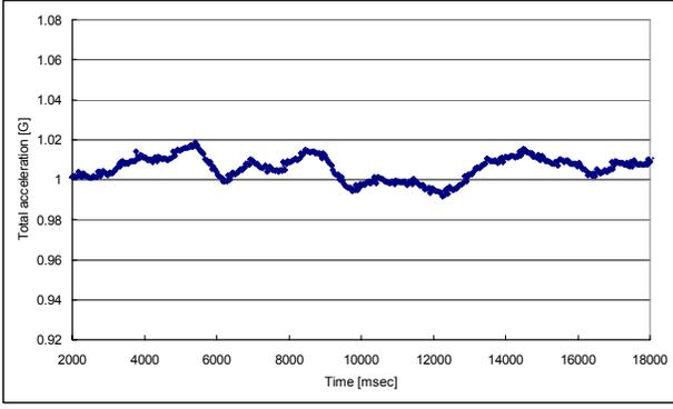
Figure 17: Example of vector length of aggressively low-pass filtered vertical acceleration vector while walking on flat floor.
