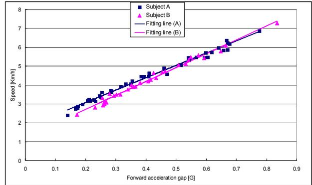
Figure 8: Relationship between forward acceleration difference and walking speed (by subjects A and B).
