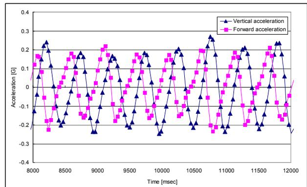
Figure 1: Typical pattern of vertical and forward acceleration walking locomotion on flat floor.
