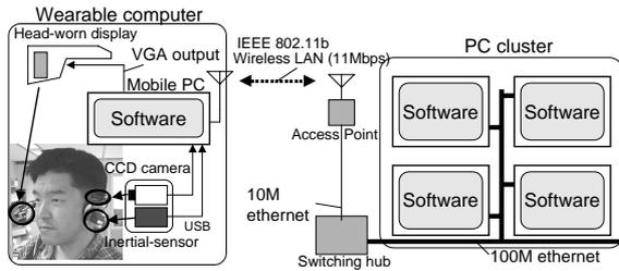
Figure 2: Diagram of our wearable vision system.
